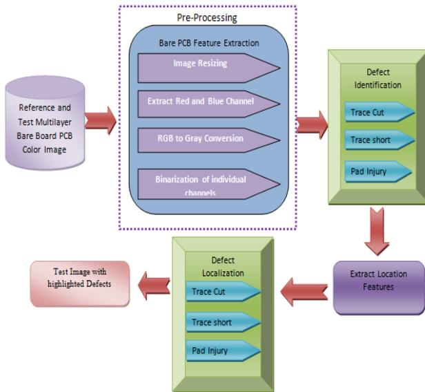
**Figure 10.** Flow of the proposed method
