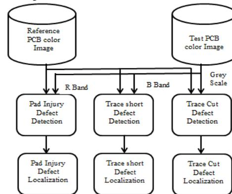
Figure 9. Block diagram of the Proposed method
