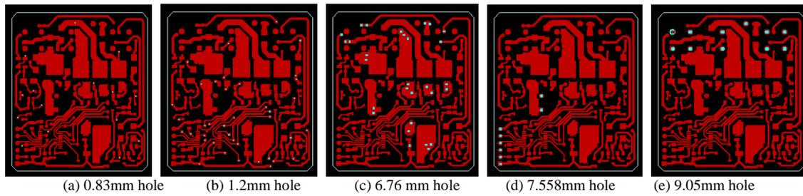
Figure 8. Through holes of different size for the Sample Multilayer PCB
