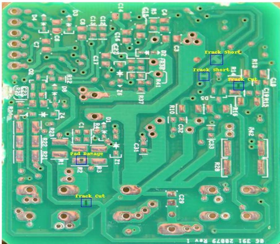
Figure 14. Localization of the defects for Bottom Layer
