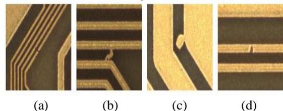
**Figure 3.** PCB image after etching process: (a) Disconnection (b) Connection (c) Projection (d) Crack
