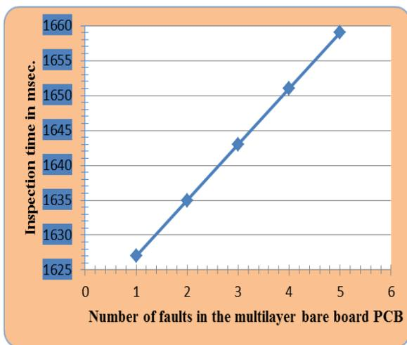
Figure 16. Time taken for the inspection board with variation in quantity of faults
