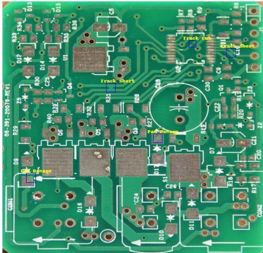
Figure 13. Localization of the defects for Top layer
