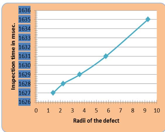
Figure 15. Time taken for the inspection of the board having only one fault with varying radii
